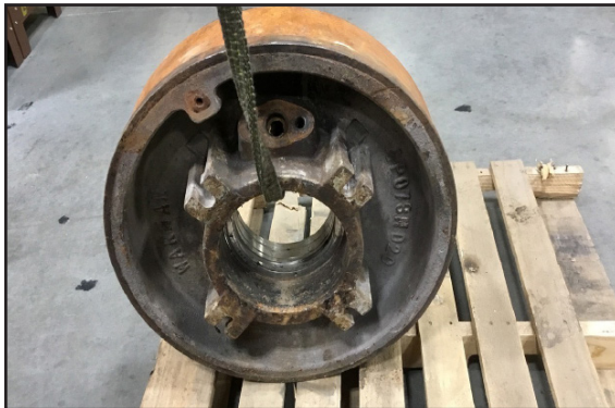
Stuffing box showing erosion and corrosion.
